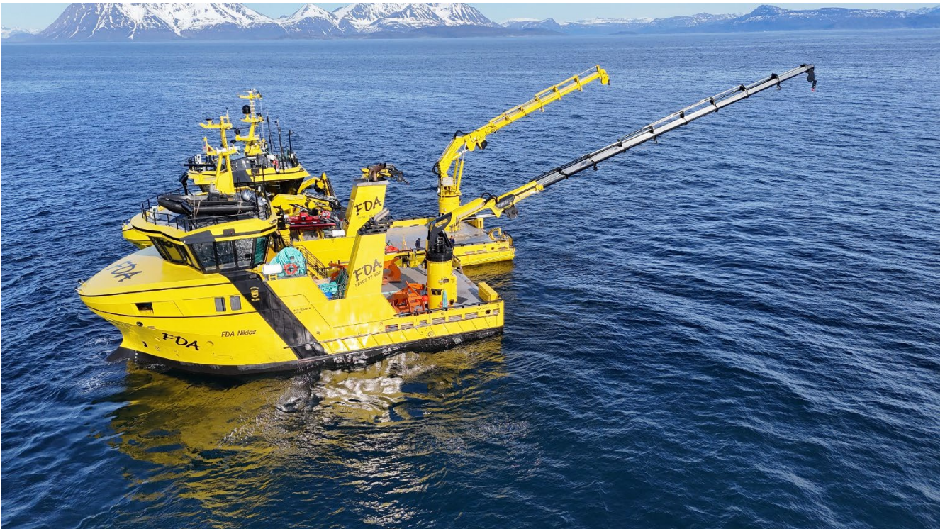
FDA vessels equipped with a combination of several PALFINGER MARINE cranes. © Tommy Grønning
